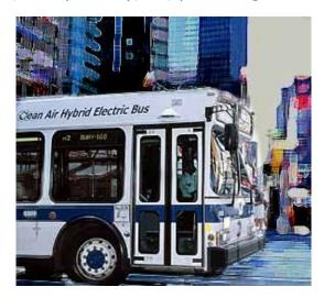
The MTA is reporting that their new Orion VII hybrid buses are making a big dent fuel consumption. Orion VII hybrid buses have improved fuel economy of more than 30% compared to conventionally powered buses. In addition, the Orion hybrids significantly reduce emissions with 90% less particulate matter, 40% fewer oxides of nitrogen, and 30% fewer greenhouse gases. The MTA estimates that they saved over 1 million gallons of diesel fuel last year.
