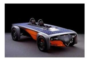
Solar Electric CarAstrolab, the world's first commercial solar car, will be available in January 2008 thanks to automobile designer Sacha Lakic. The car was developed by the French manufacturer, Venturi. The vehicle is powered by energy from the sun - the 16kW electric motor requires very little energy for propulsion. The solar hybrid can travel a minimum distance of 110 kilometres and has a top speed of 120kph.
