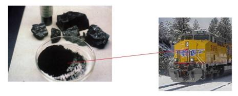
Improve the design of crushing equipment so that coal can be reduced in size to < 5 micron (where it can be mixed with water and used in diesel engines). GE has tested this in their locomotives, under DOE funding.
