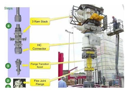
The 18-ft Lower Capping stack will now be lowered, on drill pipe, to fit on top of the transition spool. It sits on the HC connector, and is fitted with rams to control or stop the flow, and connectors that will allow feed of the oil to the different risers that will carry it from the well to the surface vessels.
