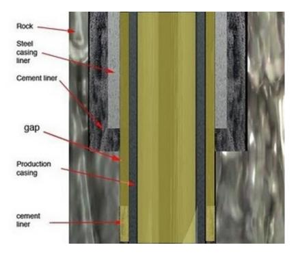
Section through the well showing with the light yellow color the channels that the oil might flow through up the well, and which will be filled with mud.
