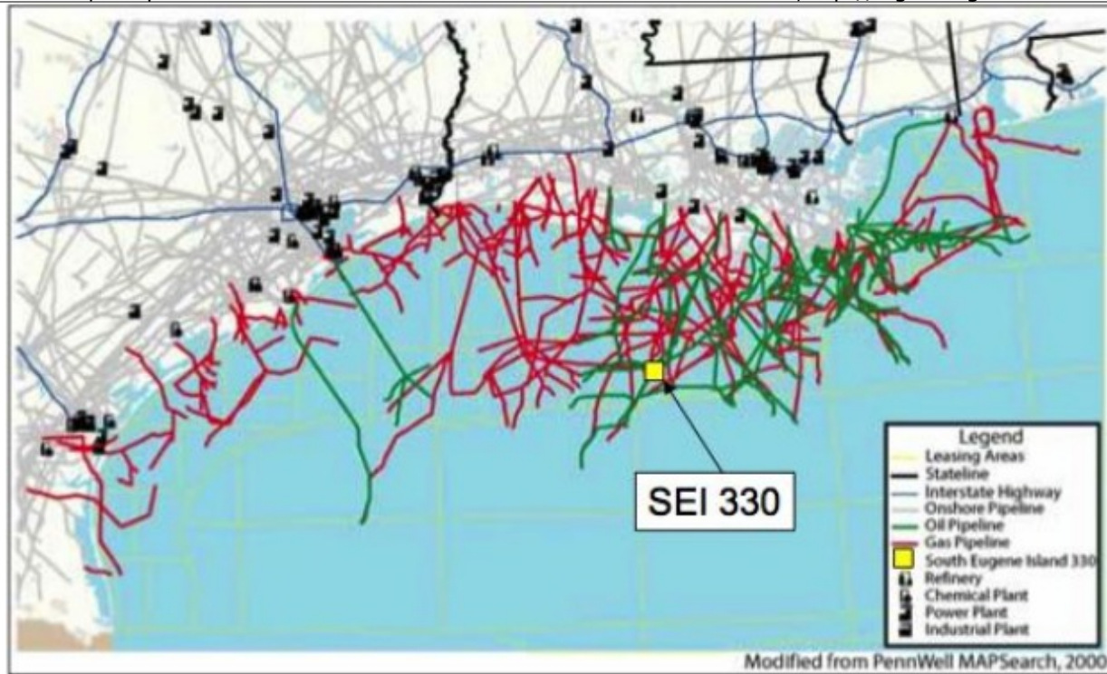
Figure 6: Map of the U.S. Gulf Coast and Gulf of Mexico and some of the existing infrastructure in the region 20 . Oil pipelines are in green, gas pipelines in red, and onshore pipelines in gray. The black figures are possible sources where anthropogenic CO 2 that could be captured and separated for sequestered in the Gulf of Mexico. In yellow is the location of our case study site, South Eugene Island Block 330.
