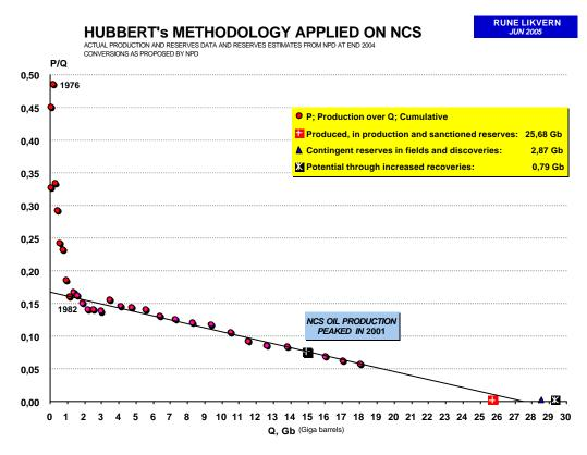
The above diagram illustrates that Hubbert's methodology would predict total recoveries of 27,41 Gb of regular oil from NCS. (For non-technical readers; that's where the sloping line intersects the x-axis (horizontal axis).)
