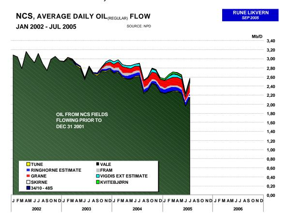
The figure above illustrates average daily (based on monthly NPD data) oil flow from NCS from January 2002 to July 2005. In the diagram new fields starting to flow post January 1<sup>st</sup> 2002 are shown with different colour coding to enhance the effects from depletion from all fields starting to flow prior to December 31<sup>st</sup> 2001.
